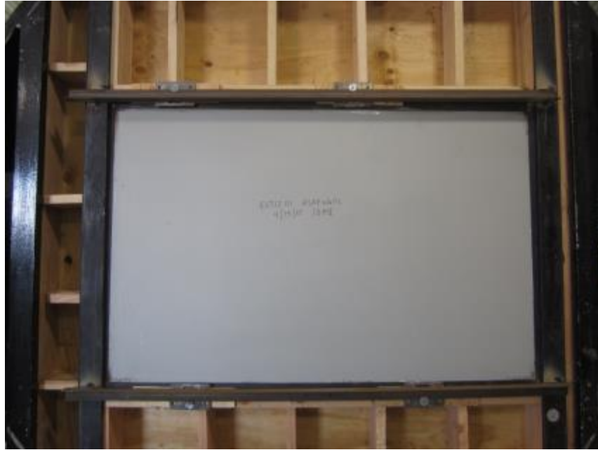
Photo No. 1 Pre-Test Condition of Wall Specimen, Interior
