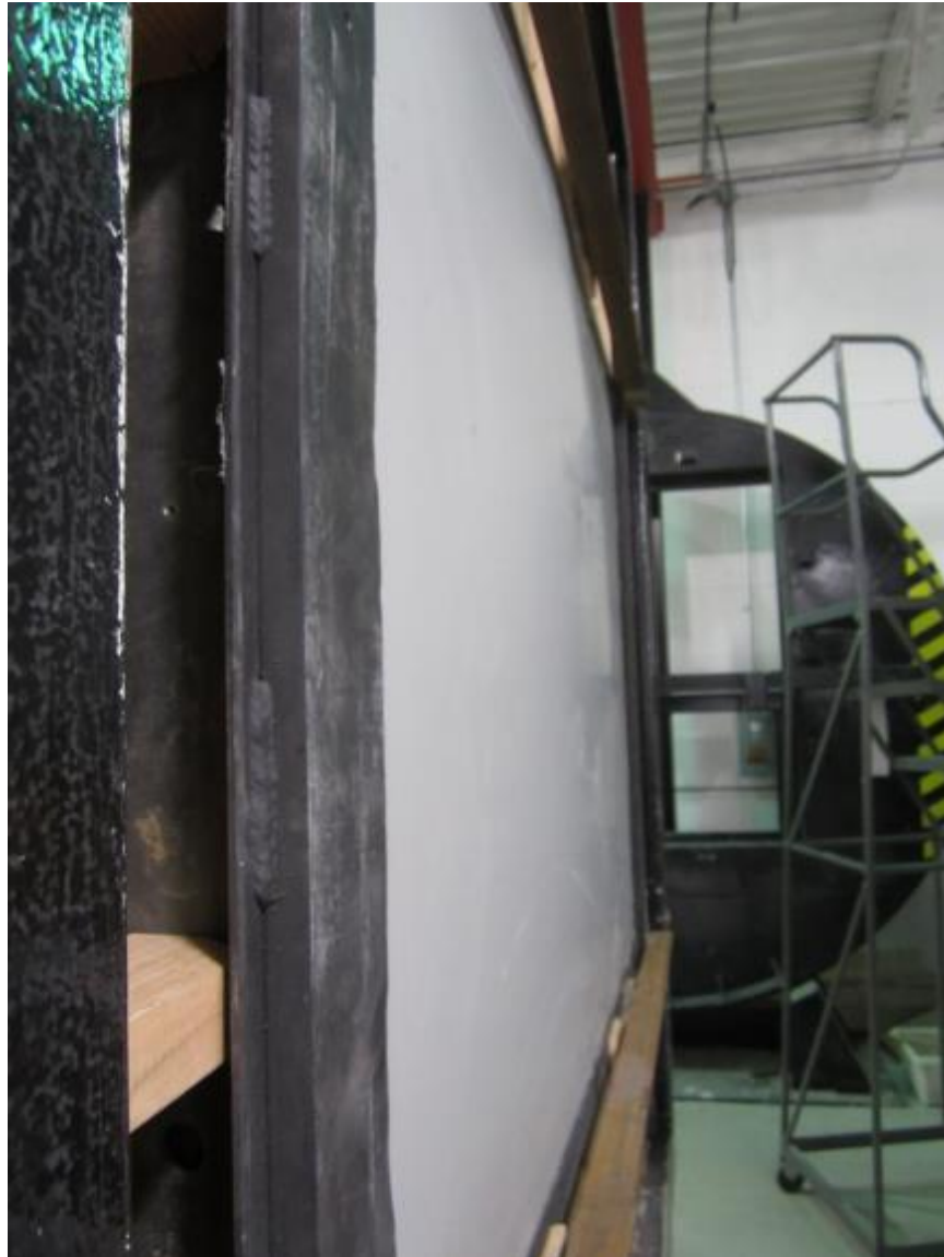
Photo No. 3 Post-Test Condition - Slight Permanent Deformation of s-Wall Panel
